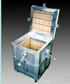
Pressure Cell Test Containment Unit
